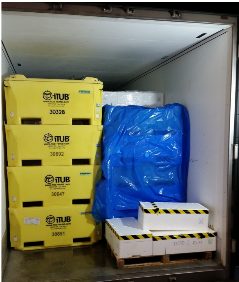
Figure 26 Sub chilled rainbow trout in container packed Sæplast tubs and EPS boxes, without ice.
