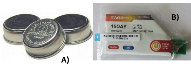
Figure 31. A) IButton DS1922L temperature loggers used to monitor the temperature within the product and the ambient temperature. B) Tempsen ITAG-PDF single use temperature logger used to monitor the temperature of product and the ambient temperature.
